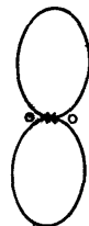
Fig.798.- Field-strength diagram of two aeri-als spaced \lambda/2 apart and fed in phase.
