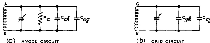
Fig. 398 - Common-cathode oscillator: effective tuned circuits.
